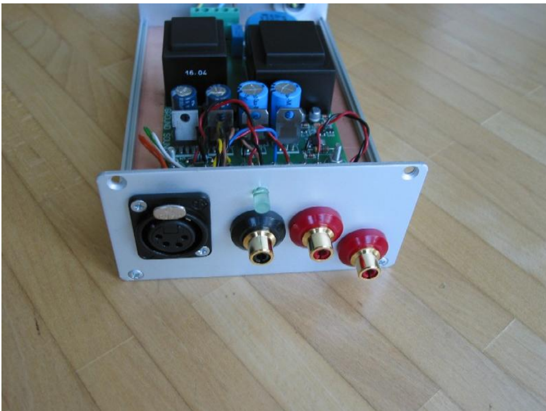
Total stack height is 47mm, free space inside the case 48mm.
