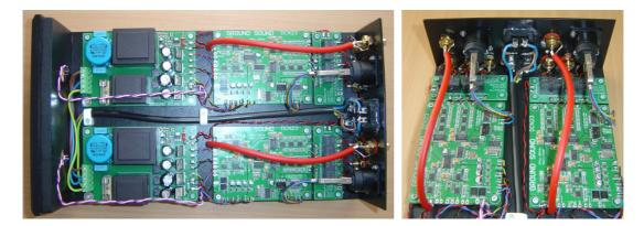
In the back plate the chinch (one input, upper one; three outputs), the USB and power (one for both PSU's with switch) connectors integrated.
