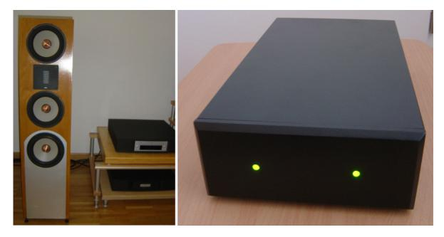
One enclosure was build for both channels left and right. Base and front made of MDF, the back and cover made of Aluminium, all parts painted black. The power LED's integrated into the front plate.
